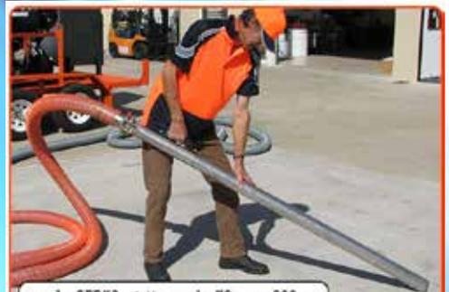
code: GPR38 - gutter probe 38mm x 800mm
